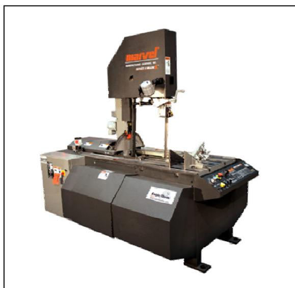
Made by MARVEL, vertical tilt-frame band saw SERIES-8
